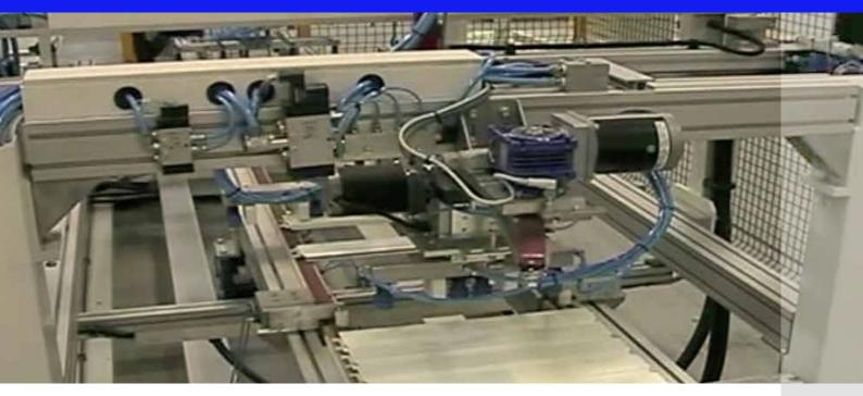
This machine is designed for assembling of inside doors and kitchen doors in wood or MDF, with 90° or 45° junction, and the possibility to have one or more panels both wood or glass.
