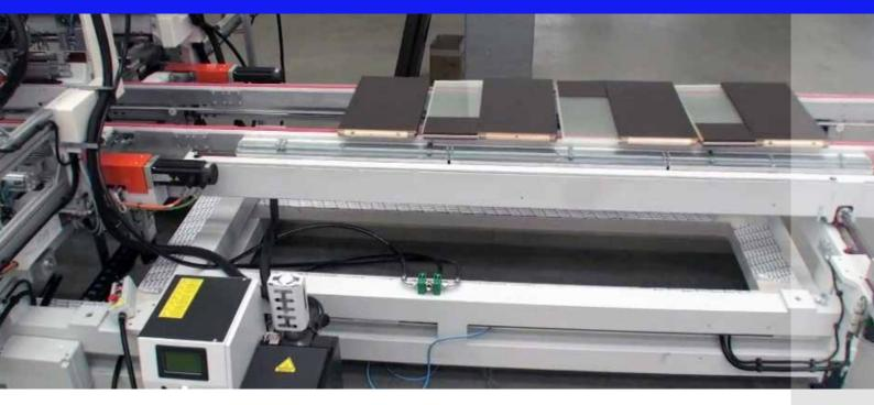
This machine is designed for assembling of inside doors in wood or MDF, with 90° junction, and the possibility to have one or more panels both wood or glass. The combination of vinilic and hot melt glue allow to have at the output of the machine a door perfectly fixed ready to be packed. Every mechanical parts and relative dimensions change could be completely automatic.
